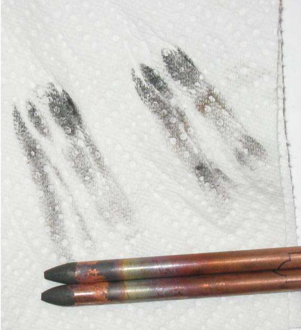
Prior to conducting a Vreeland spectroscopy burn the copper-coated carbon arc electrodes are sanded and wiped clean with a paper towel to remove any potential contaminants from previous use.
